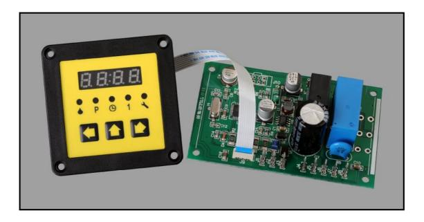
Universal Control Unit UC-1A is designed for controlling and monitoring of centralized lubrication systems. It is widely used in lubrication system control for automobile chassis, construction machinery and small machinery and equipment
